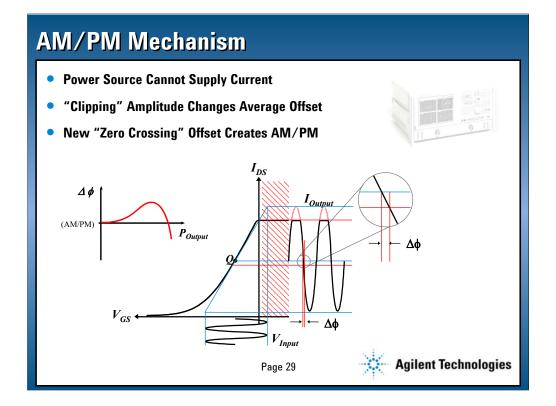
The phenomena that gives rise to AM/PM again begins with the power source limitation creating a clipping or "mushing" of the waveform. Since the top of the waveform is not correctly amplified, the average value or "zero crossing" is offset from the original position. This offset in "zero crossing" occurs where the sine wave has finite slope creating a phase shift in the output signal.
