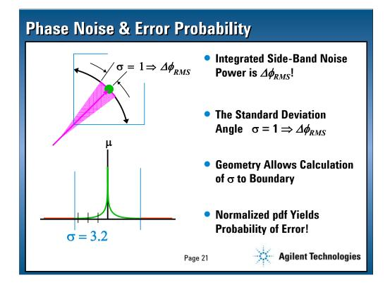
Integrating side-band noise power over the appropriate limits gives us the RMS angular phase noise in degrees ( $\Delta\phi_{RMS}$ ) that will effect the modulation.
