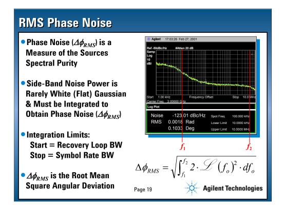
So how does one characterize and account for phase noise in the probability model? First, we must understand that phase noise is a measure of the source's (local oscillator's) spectral purity or how perfect the sine wave is produced.
