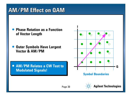
The AM/PM phase shift as a function of signal amplitude or vector length distorts the ideal symbol location of the QAM symbol constellation.
