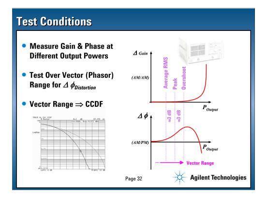
What test conditions are necessary to properly characterize the distortion of the power amplifier? The gain and phase distortions need to be characterized over the range of modulation powers. This means that AM/PM should be tested from the smallest vector needed to produce the modulation, to the largest vector or in other words, over the "vector range."
