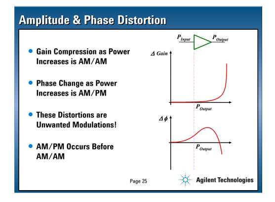
To predict residual BER, linearity metrics that directly relate to the QAM vector in amplitude and phase are needed. Gain compression or the difference between the ideal linear gain and the actual gain is amplitude modulation due to amplitude modulation conversion (AM/AM).
