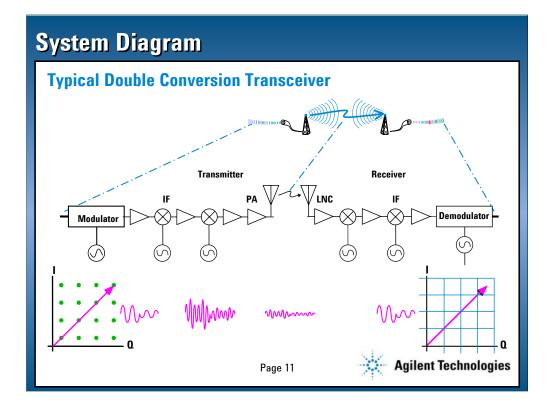
In the typical digital radio, bits come to the modulator and are mapped to a symbol point. The vector is then driven to that symbol point.
