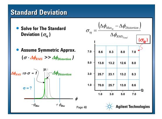
The previous equation can be solved for sigma  $(\sigma_{iq})$  for each of the constellation points. It can easily be seen that the number of sigma to the boundary is much lower for the outer states than for the ones close to the origin. This means that virtually all the residual errors occur in the outer most symbol points.
