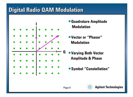
Most modern digital radios use QAM or some form of it. QAM stands for Quadrature Amplitude Modulation which is a vector modulation or Phasor modulation. It is created by taking two vectors which are 90 degrees apart and amplitude modulating them, then summing them together to from a resultant vector. The resultant vector can be modulated in both amplitude and phase.
