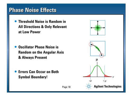
The preceding discussion was for a simplified random noise model often found in textbooks for the analysis of threshold noise. This model is the basis for threshold effects which are random in all directions and only relevant at low power.
