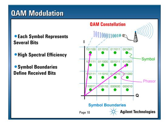
Each symbol represents several bits, allowing more information to be sent with each sample of the vectors position. [Note: Only a signal quadrant of the constellation is shown!]
