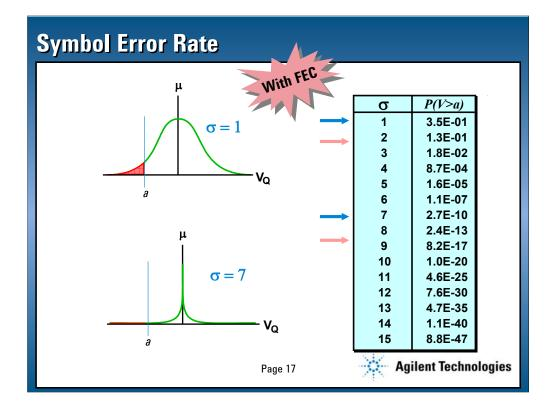
Counting the number of standard deviations to the symbol boundary provides a means to determine the probability of a symbol error.
