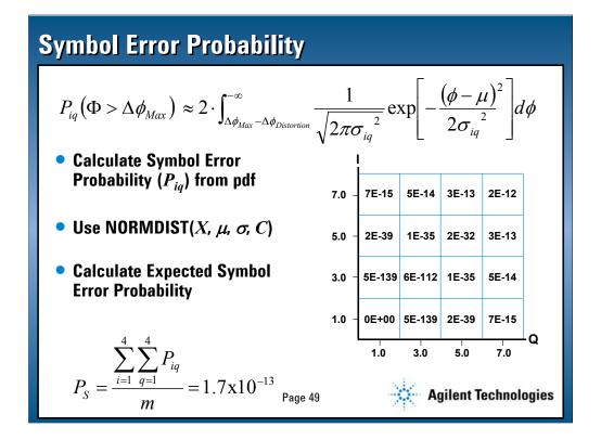
The number of sigma's to the boundary enable the use of the normalized probability density function (pdf) to calculate the probability of each symbol error  $(P_{ia})$ .
