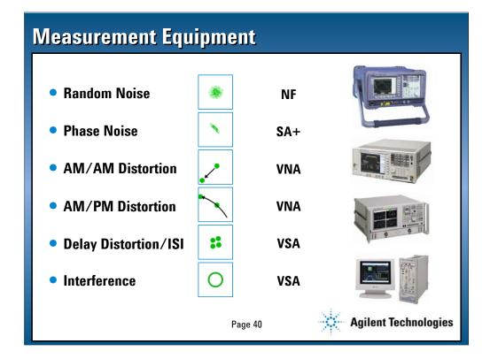
There are many approaches to measuring the different error mechanism types. The most common solutions are shown on this slide, and of course Agilent offers a complete portfolio of equipment.
