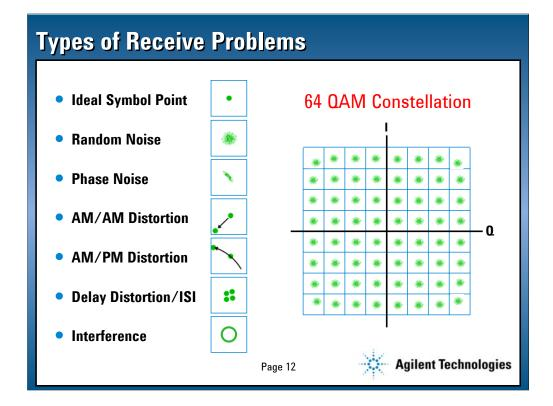
Ideally, at the receive demodulator a single infinitesimally small sample point would be found in the center of the symbol boundary area. Unfortunately, this never occurs because there is always noise, distortion and interference components present.
