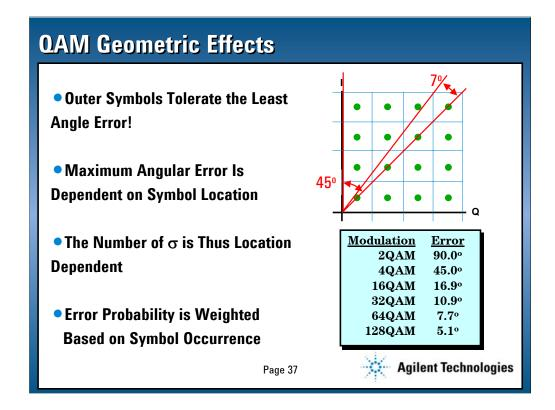
The QAM symbol constellation has some important geometric effects to consider. The outer symbol points can tolerate the lease angular error. In the 64QAM constellation the outer most point can tolerate a maximum of 7.7° of error before making a symbol decision error versus the inner most point which can tolerate 45° of error. The outer most point also has the longest vector length and corresponding highest angular distortion.
