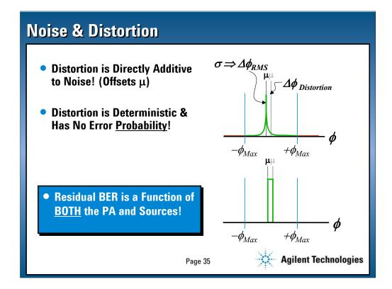
Distortion is directly additive to the noise because it operates on the vector itself. This has the effect of offsetting the mean value of the probability density function.
