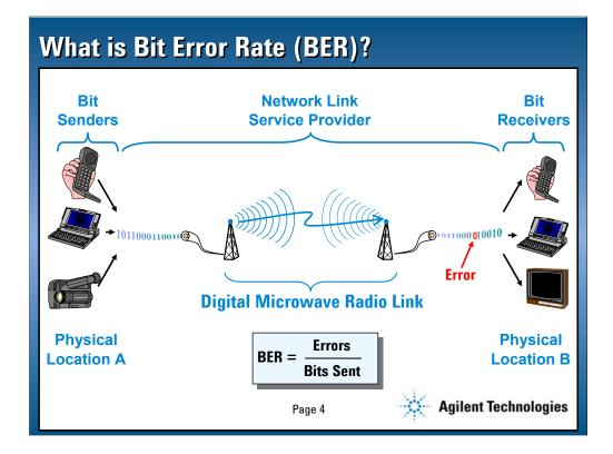
In any digital communications link there are bit senders and bit receivers that are physically separated. These devices are linked together through a network link, often provided by a third party service. The network links can be wire, coaxial cable, fiber optic, microwave or some combination.
