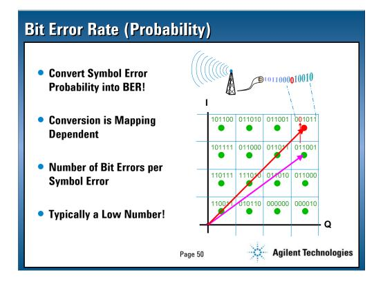
The symbol error probability must now be converted to the bit error rate (BER) or probability of a bit error. The conversion of symbol errors to bit errors is bit mapping dependent (i.e. the arbitrary assignment of six different bits to each symbol in the constellation).
