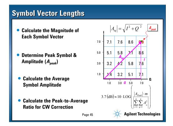
First, using Pythagoras's theorem calculate the magnitude of each symbol vector in the constellation. Using symmetry the work can be simplified by only calculating a single quadrant.
