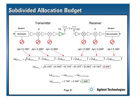
If the calculated BER is acceptable no reallocation of distortion or phase noise is necessary. The final step is to subdivide the total allocation into the components of the system which generate it.
