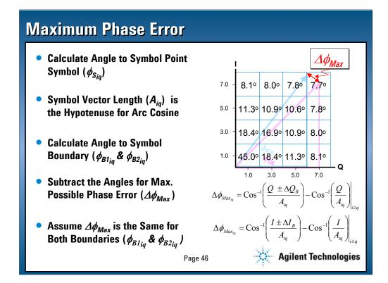
Using the constellation geometry, the maximum permissible phase error to the symbol boundary can be calculated. Begin by calculating the angle to the symbol point  $(\phi_{iq})$  using an arc cosine relationship and realizing that the symbol vector length previously calculated is the hypotenuse of the triangle.
