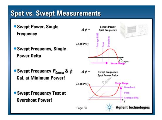
There are two types of AM/PM measurements, spot and swept. The classical diagram of AM/PM or  $\Delta\phi$  versus power level, often seen in linearizer work, is a spot frequency versus swept power measurement. This measurement is best suited for fixed frequency operation since the matching, hence AM/PM, is usually a function of frequency.
