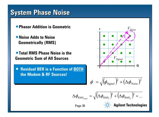
System phase noise can be represented by a noise vector which adds geometrically to the desired modulation vector. Noise from more than one source can be added geometrically to obtain the total noise for the system.
