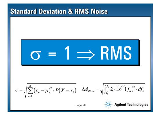
A key relationship essential to realize is, that the one sigma distance happens to be identical to the RMS error!!! Often statistics courses are taught in such a way that connection between RMS and sigma are never clearly stated to the engineer.
