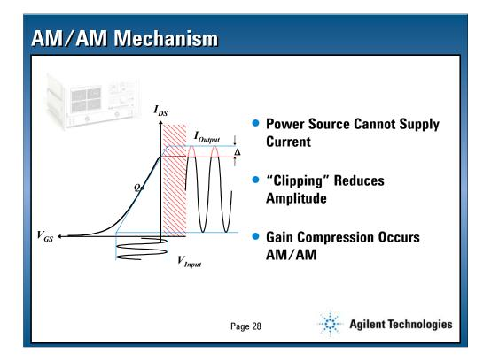
The AM/AM mechanism is very simple to examine with our amplifier model. If we put a single sine wave into the amplifier and the power source cannot supply the necessary current resulting in clipping the amplitude of the output is reduced. This reduction is gain compression or AM/AM.
