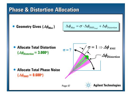
The geometry of the constellation locks down the maximum angular error ( $\Delta \varphi_{Max}$ ). The angular error is composed of a distortion component and some number of sigma times the phase noise component (neglecting other possible error sources, generally a good assumption). Next, an allocation of the distortion component and phase noise component must be made.
