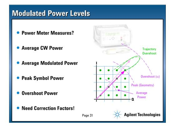
So how does one relate the vector length to known traceable standards? And what range of vector lengths do we need to measure the distortion over?
