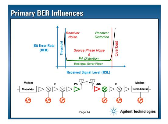
Each of these sources of constellation problems has a unique impact on the BER performance. At threshold, receiver noise dominates the BER error mechanisms. At overload, receiver distortion, primarily in the first mixer, dominates the BER error mechanism. The residual error floor is dominated by a combination of the phase noise from all the sources and the PA's distortion!
