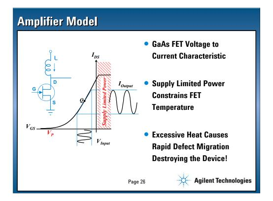
Sometimes it is helpful to review the mechanisms that actually generate these unwanted distortions in the power amplifier. Let's use a simple GaAs MESFET model to illustrate the principles. To keep it simple we have omitted the effects of microwave matching circuits that are of finite bandwidth and linear in nature.
