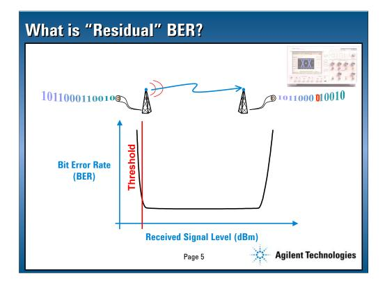
What is "Residual" BER? In a microwave data link bit error rate is a function of the Received Signal Level (RSL) sometimes called Received Signal Strength (RSS).
