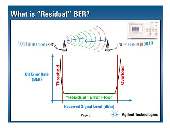
As received signal strength increases, the error rate will fall to a very low level or error floor. This error floor is called the "Residual" bit error rate or "Residual BER". It is the 'normal' operating performance of the data link.
