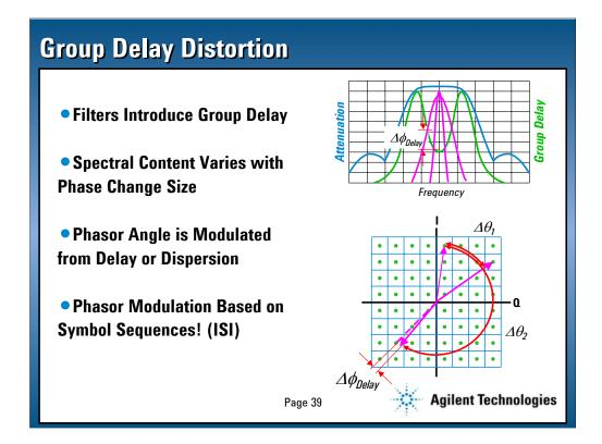
Filters introduce group delay into the modulated channel. The spectral energy associated with a change in phase is dependent on the magnitude of phase modulation. Small changes in phase occupy small bandwidths, large changes in phase occupy larger bandwidths.
