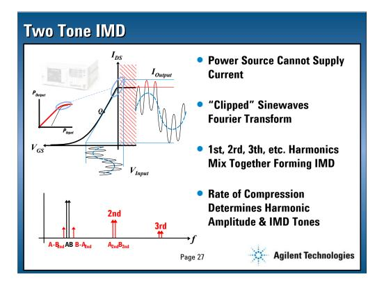
In a two tone IMD test, identical amplitude tones separated slightly in frequency are injected into the input of the amplifier. The power supply cannot deliver additional current so the superimposed sine waves are "clipped." This gives rise to 2nd, 3rd etc. harmonics which mix together forming the IMD products.
