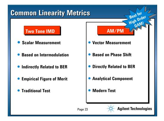
Commonly used linearity metrics are, two tone intermodulation distortion (IMD) testing and amplitude modulation to phase modulation conversion testing (AM/PM). Let's review each briefly.
